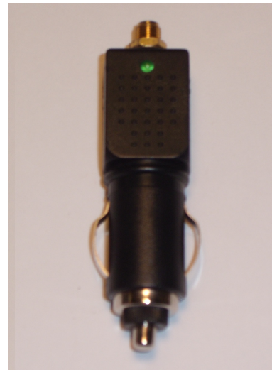
Figure 7 Cigarette Lighter Jammer, Group 1, with antenna removed.
