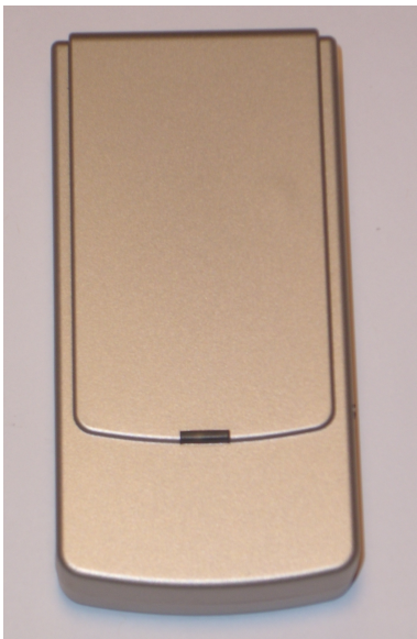
Figure 14 NonSMA-Battery Jammer, Group 3. It is meant to be disguised as a cellphone.
