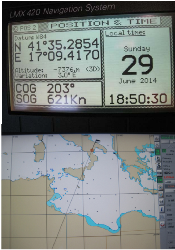
Fig. 14. The WROD bridge GPS receiver display (top picture) and its GPS-driven chart (bottom picture) during the Libya spoofing scenario.
