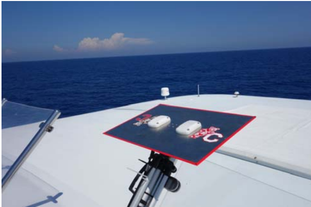
Fig. 8. The two antennas of the prototype spoofing detection system mounted on a common ground plane.
