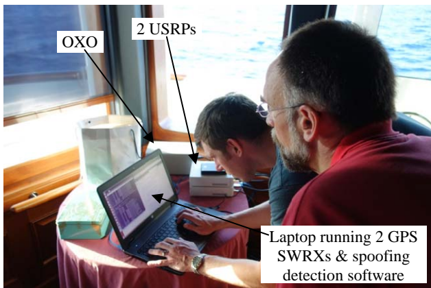
Fig. 9. Signal processing hardware of the prototype spoofing detection system.
