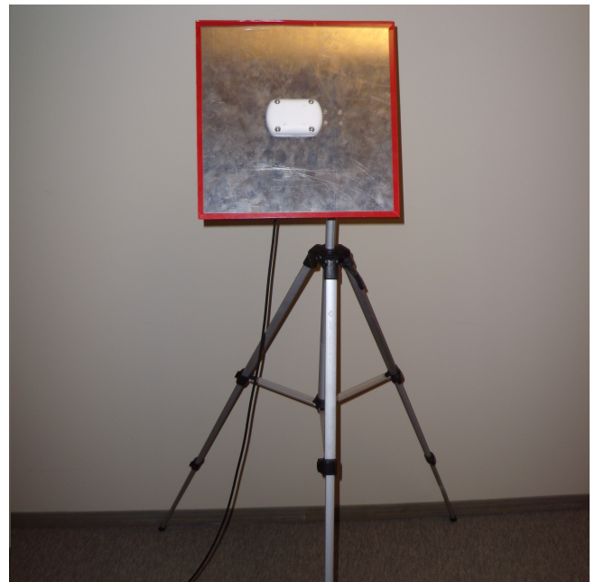
Figure 16 Jammer pickup antenna on ground plane, mounted on a tripod for easier aiming.
