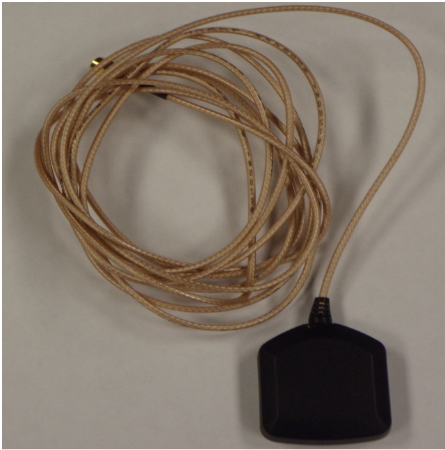
Figure 17 GPS pickup patch antenna. Mounted on a large ground plane and shielded with a car when used in the field.
