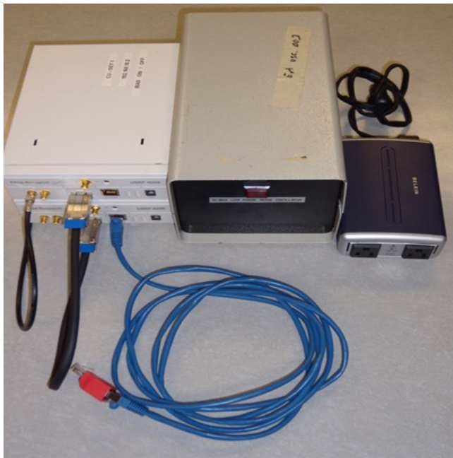
Figure 15 General purpose RF recording equipment. The two boxes on the left are Ettus Research USRP N200s, the box in the middle is an ovenized crystal oscillator and the box on the right is a power inverter.
