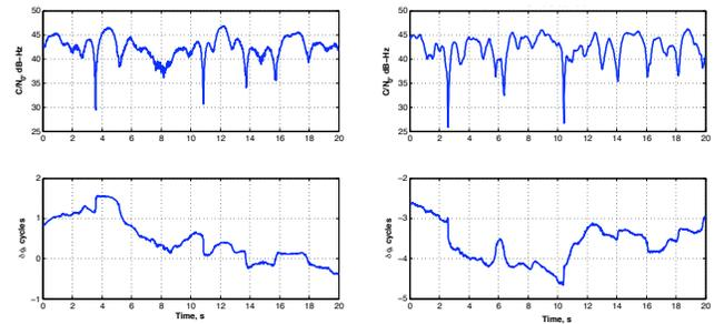
Figure 9. A comparison between empirically-derived scintillation data (left) and simulated scintillation data (right).
