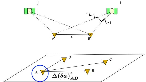
**Figure 5.** The relative navigation scenario with one satellite scintillating (top) and the phase relationships in the scintillation imaging array (bottom).
