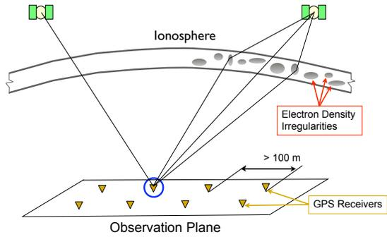
**Figure 1.** The undisturbed and disturbed ionosphere and the scintillation imaging array.
